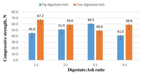
Fig 1. Average breaking force of granule in longitudinal direction in dependence on digestate: ash ratio
